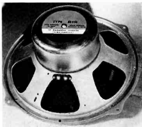
Fig. 5—Photograph of the back of the duo-cone loud speaker mechanism Type 515S1.
